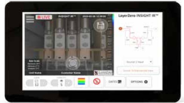
INSIGHT IR® live images can be viewed on a local or remote display.
