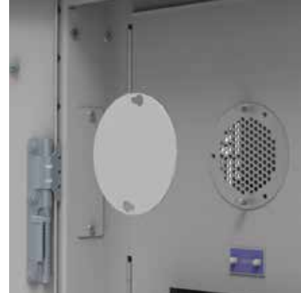
INSIGHT IR® Portholes allow operators to safely scan bolted connections without opening the dead front doors
